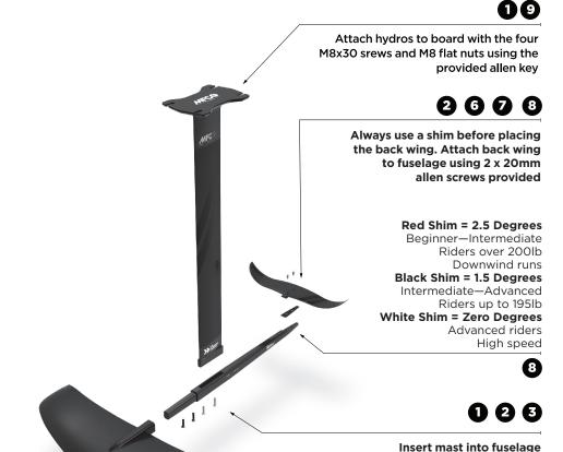
Insert front wing into fuselage attach by using the 2 x 20mm allen screws provided
